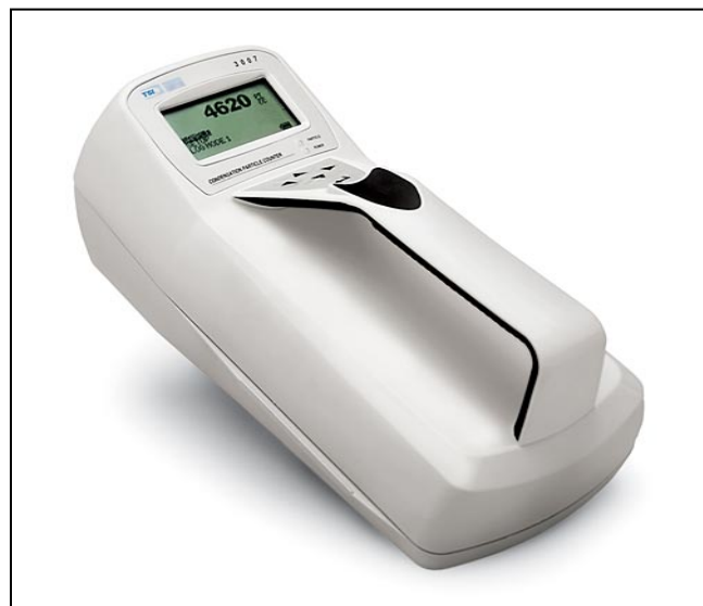
Figure 4.9 TSI Model 3007 Condensation particle counter (CPC).
