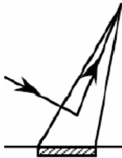
Figure 35: Radiation received at the sensor due to scattering from the atmosphere (Vermote et al. 2006)
