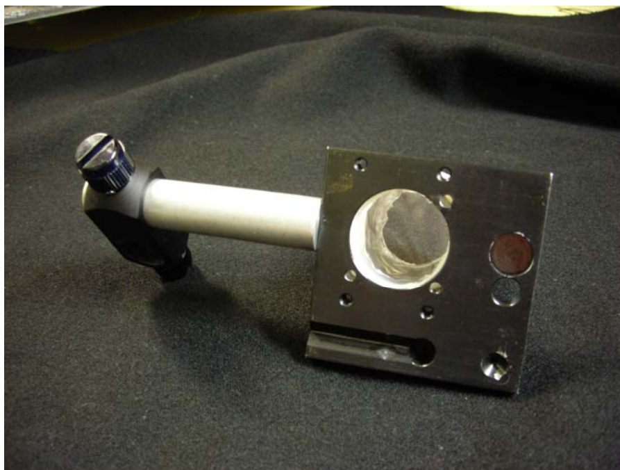
Figure E.2. Teflon sample holder for 90° scattering measurements
