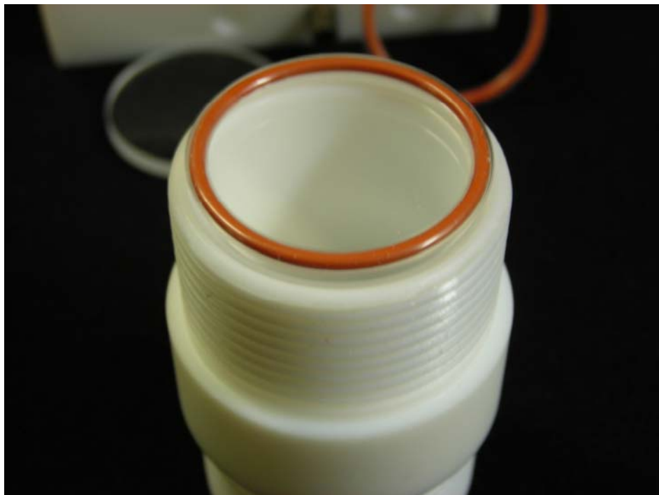
Figure E.4. Close-up of Teflon sample holder with Teflon coated O-ring
