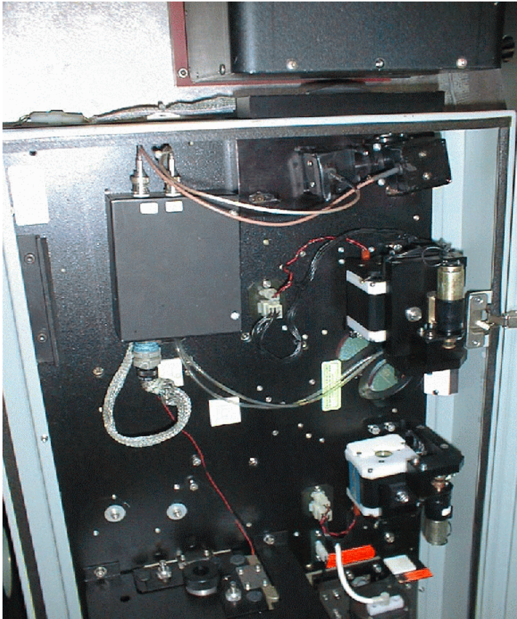
Figure 3.3. LAPS Transmitter optics [photo credit, C.R. Philbrick].
