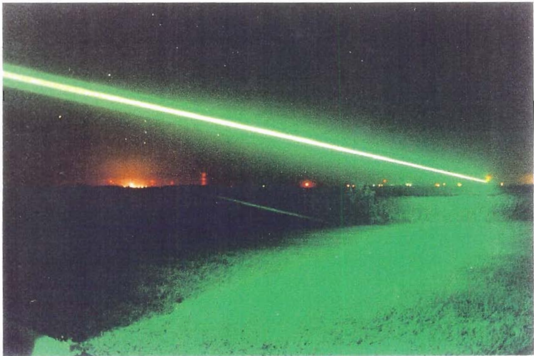
Figure 3.5. This photograph shows what the bistatic receiver sees on a clear night. The bright spot at the end of the laser beam is the target board.
