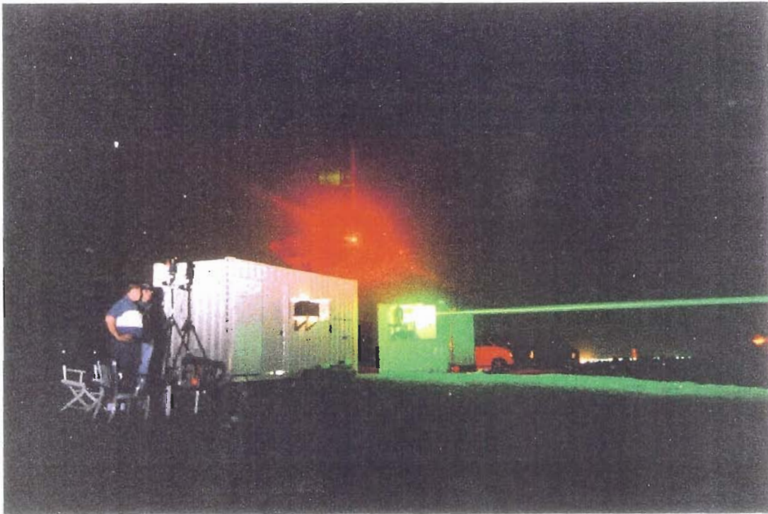
Figure 3.4. A photograph of the laser propagating toward the target board. The bistatic receiver can be seen located next to the white office container.
