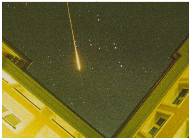
Figure 2: Photograph of a self-guided filament induced in air by a high-power, infrared (800 nm) laser pulse [16].
