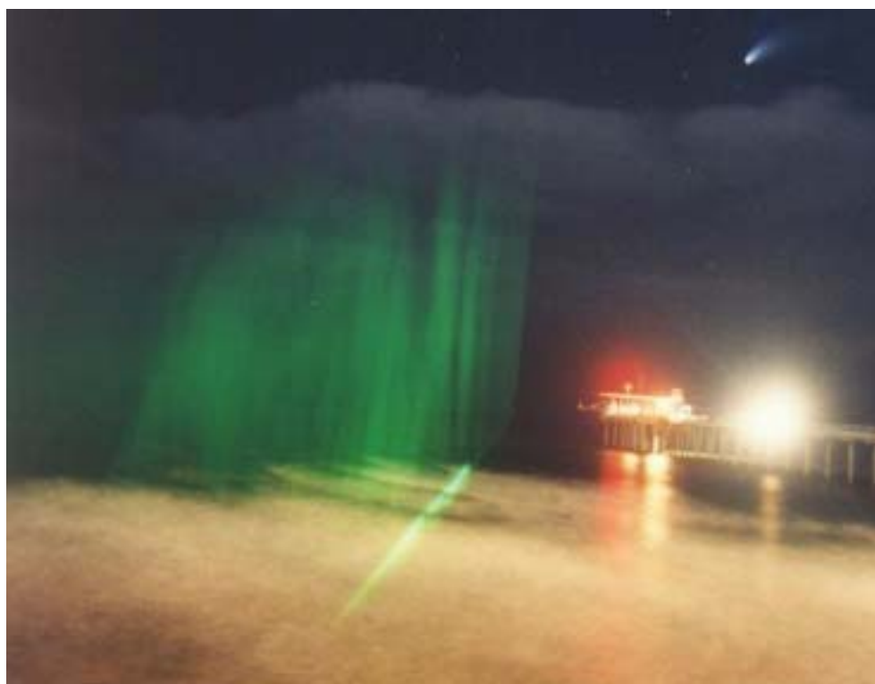
Figure 1. Representative sample of surf-zone plumes taken at the Scripps Institution of Oceanography (La Jolla, CA) when illuminated by a vertically fanned argon-ion laser. (Photo by C. R. Philbrick.)
